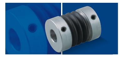
Bellows couplings that use a plastic (polyester resin) boot with plenty of elasticity in order to achieve high damping performance and extremely small counterforce from mounting misalignment. A compact design that unitizes an aluminum alloy hub and plastic boot means there is no backlash.
